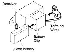
Figure 48 - Installing Battery in Receiver
